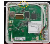
The Upper center boss for fixing the bent cable
